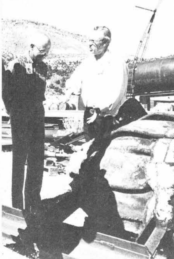
"THIS FAC [fast-acting closure] shuts off a 30-inch hole in a thousandth of a second," Carter Broyles explains to Welber. FAC and other Sandia-developed closure systems play a key role in underground nuclear tests.
